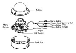
Figure 1. 1 Overview of TVIVFDIR120 Outdoor Dome Camera
