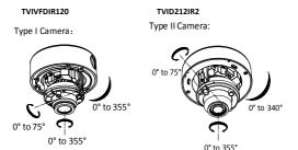
Figure 2. 4 3-Axis Adjustment
