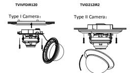
Figure 2. 6 Fix the Camera to the Mount
