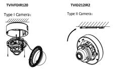
Figure 2. 3 Fix the camera to the Ceiling
